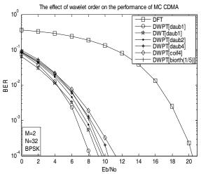
Figure 8. BER vs. Eb/No of DWPT Based MC-CDMA in the AWGN Channel [8]
