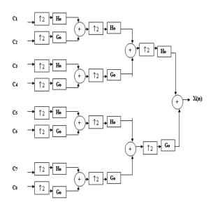
Figure 2: Three levels of wavelet Packet reconstruction tree.
