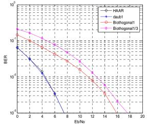
Figure 6: The BER vs.  $E_b/N_o$  performance of MC-CDMA BASED DWT in the AWGN channel.
