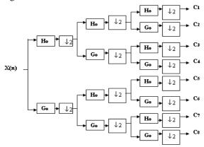
Figure 1: Three levels of wavelet Packet decomposition tree.
