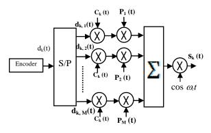
Figure 3: Transmitter Model.
