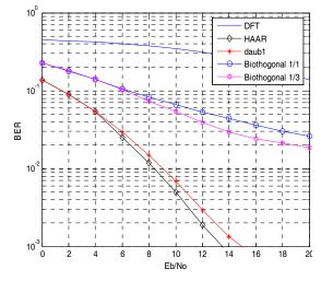
Figure 7: BER vs.  $E_b/N_o$  performance of MC-CDMA Based DWT in the Rayleigh Fadding channel.
